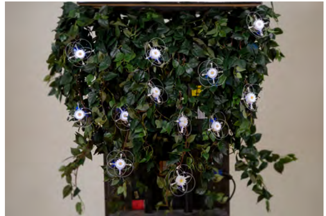
Figure 4: The drones dock to charging points integrated in a vine, which complements their floral design.
